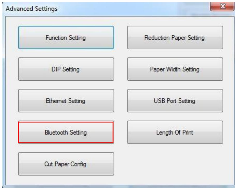
15. User can type a new Bluetooth name and password in the following window, click "set", and restart the printer to take effect of the setting.
